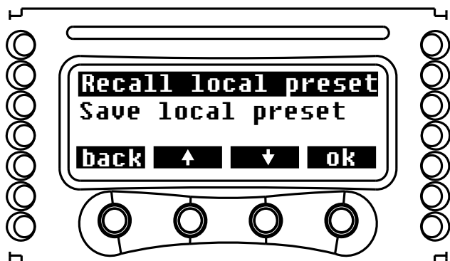
APPENDIX FIGURE 3: The main SmartCard menu is visible when the card is inserted in the amplifier's frontal slot
