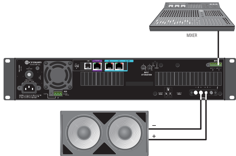
Figure 21 System Wiring Bridge Mode
